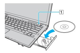
bo not exert pressure on the drive tray. Be sure to hold the bottom of the drive tray when placing/removing a disc onto/from the tray.
